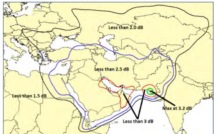
Figure 4: Coordinated Uplink Power Density & ASI Levels on IS-20 at 68.5°E from Antennas Operating on E70B at 70.5°E
