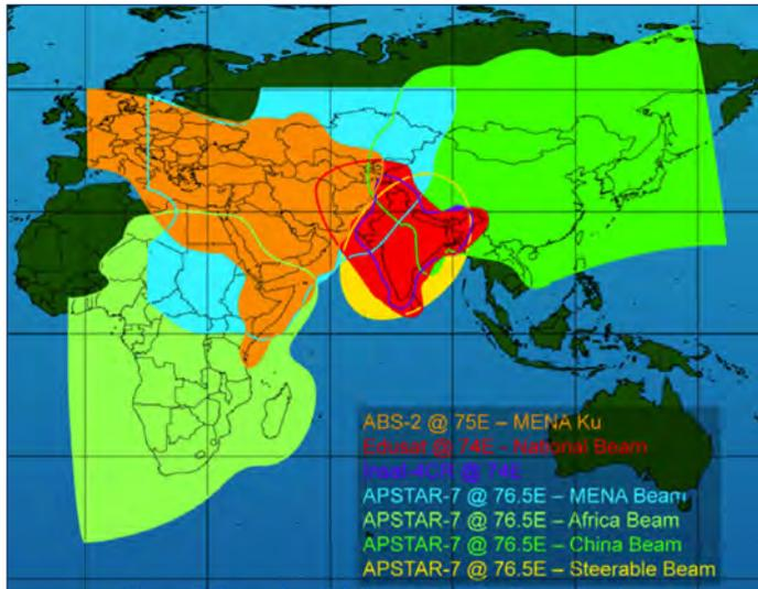
Figure 3: Examples of Adjacent Satellite Beam Overlap
