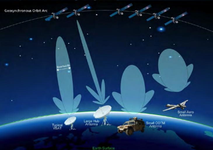
**Figure 1: Smaller Antennas Receive & Cause More ASI**
